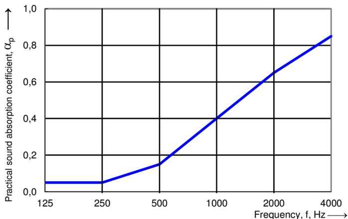
Weighted sound absorption coefficient according to ISO 11654
